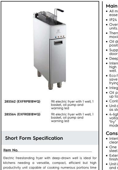
Electric freestanding fryer with deep-drawn well is ideal for kitchens needing a versatile, compact, efficient but high productivity unit capable of cooking numerous portions time after time. The well layout, heating elements layout and the "eco" mode, require a minimum amount of oil and guarantee long oil life. Made in stainless steel. 4-position tilting elements to ease cleaning and use. Oil pump.
