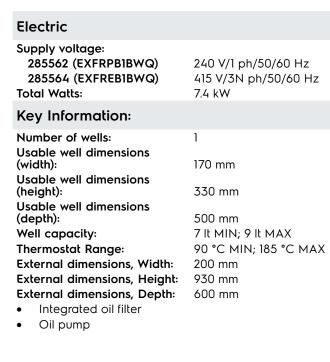
Modular Cooking Range Line 200 mm - 1 Well Electric Fryer 9 liter with oil pump
