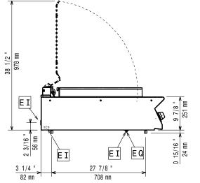
D = Drain EI = Electrical inlet (power)
