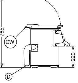
CWII = Cold Water inlet I D = Drain EI = Electrical inlet (power)
