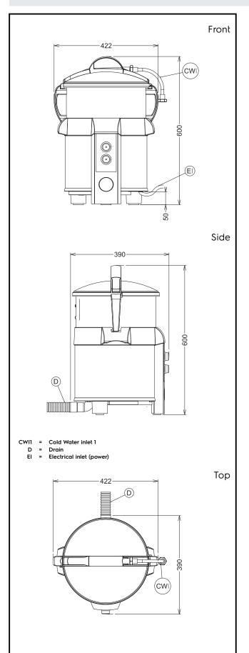
Electric Supply voltage: 601302 (T5EFB) 220-240 V/1N ph/50/60 Hz Capacity: Performance (up to): 80 - kg/hour Capacity: 5 kg **Key Information:**
