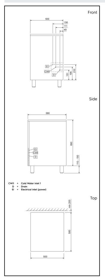
Electric Supply voltage: 730160 (FGC33AS42) 220-240 V/1N ph/50 Hz Electrical power max.: 0.37 kW Capacity: Bin capacity: 16 kg **Key Information:** External dimensions, Width: 500 mm External dimensions, Height: 690 mm External dimensions, Depth: 580 mm Output: 33 kg/day Ice Cube 42 g Kind of cube:
